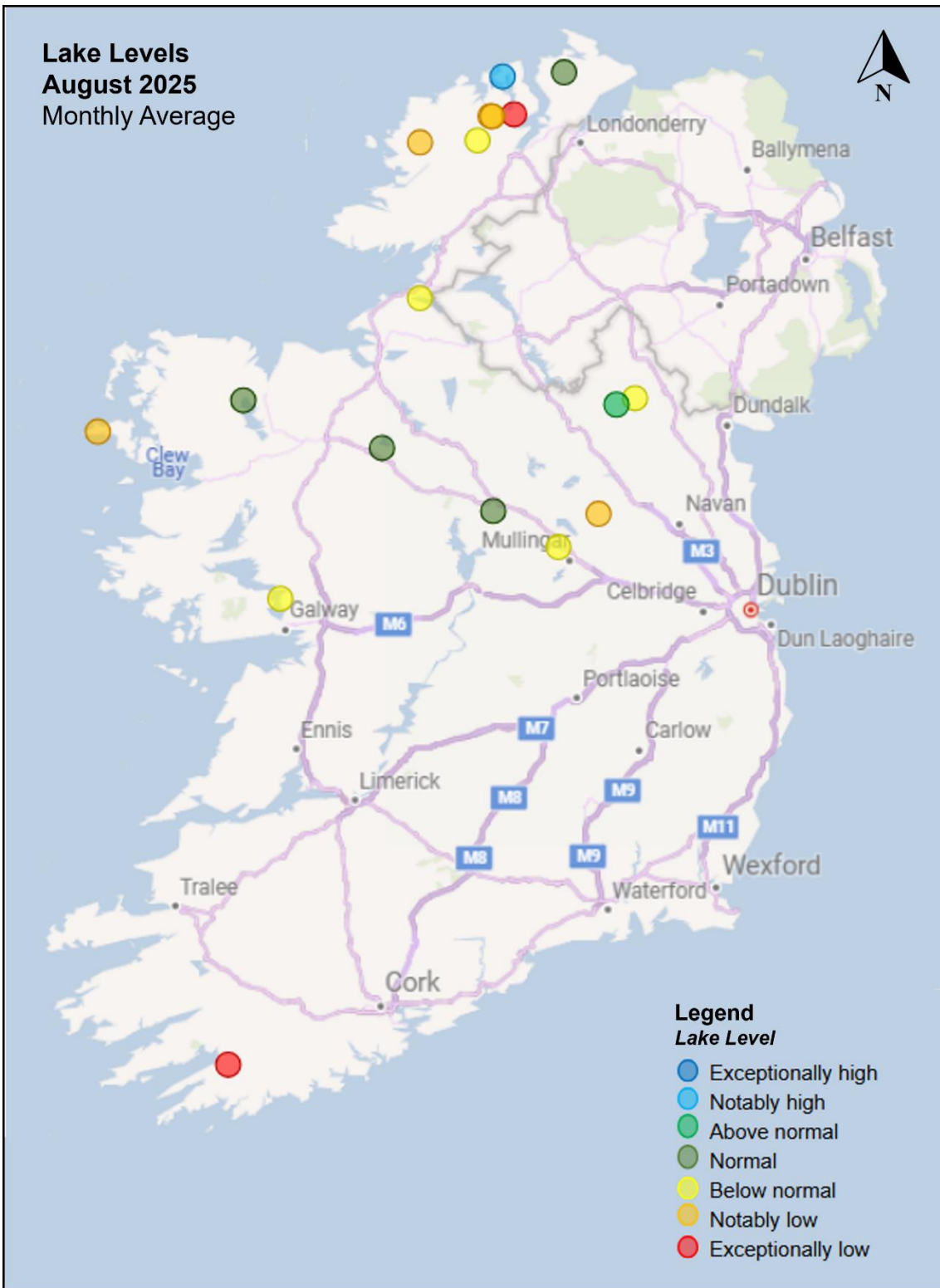
Figure 9 - Lake Levels as of August 2025. Level class based on Weibull ranking, with lower ranks indicating lowest lake levels on record for selected month.
