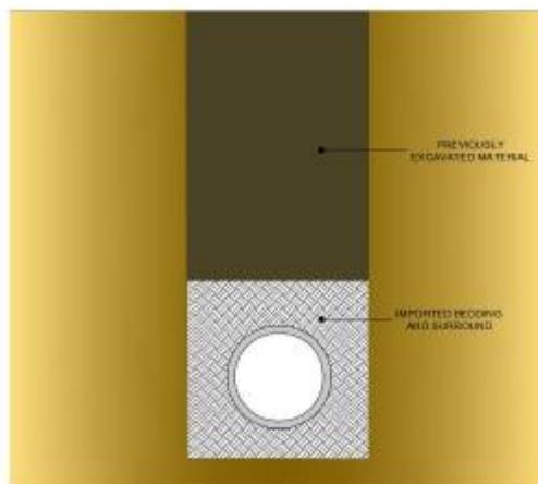
**Diagram 20.3: Bedding and Surround Imported and Trench Backfilled**
