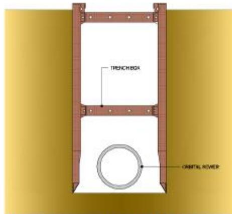
**Diagram 20.2: Trench Box Installed and Pipe Laid**
