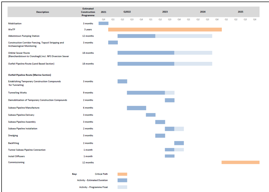
Diagram 7: Outline Construction Programme for Orbital Sewer, Abbotstown Pumping Station, WwTP & Outfall Pipeline
